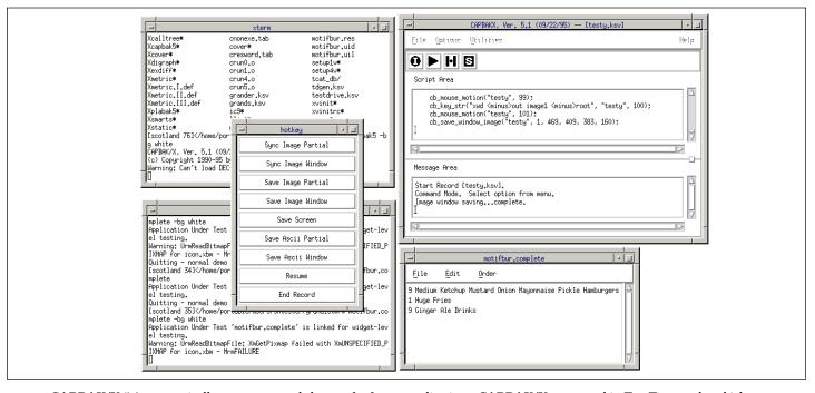
**CAPBAK/X 5.1** automatically executes recorded tests of software applications. **CAPBAK/X** can record in TrueTime mode, which reproduces precisely all GUI interactions and is sensitive to slight changes in the application, and in ObjectMode, which activates widgets directly and tolerates minor changes in the application under test.
